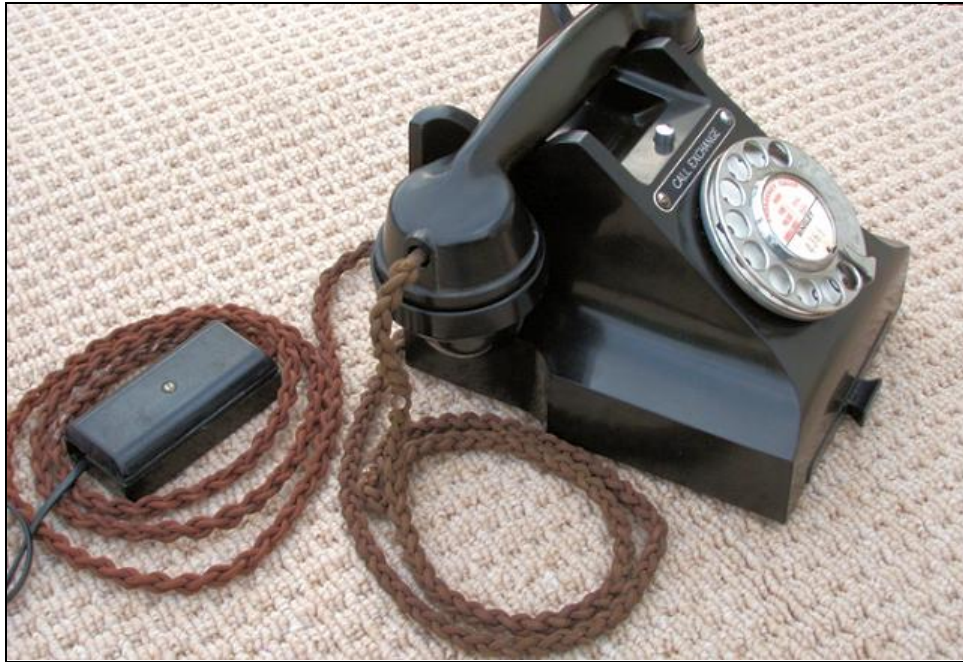
A 1950s GPO Telephone with a call exchange button Image courtesy of The Telephone Box
